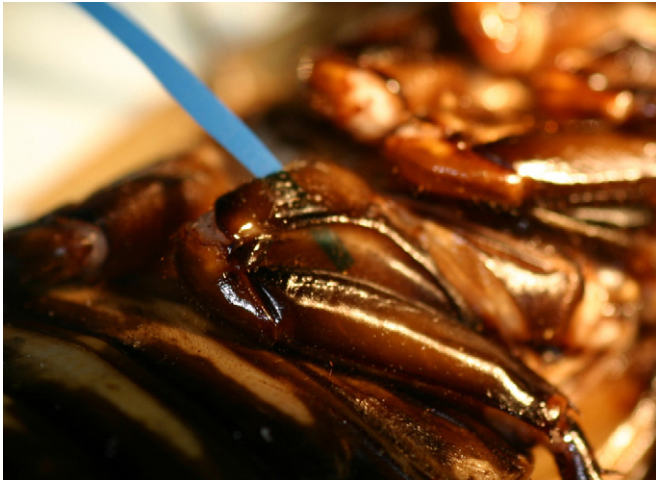
Fig. 3. Insertion of fMEAs into coxa. An opaque sham electrode illustrates the position of the fMEA, and can be seen through the cuticle, inside the coxa. Devices are sandwiched between the inside surface of the cuticle and muscles in the coxa. Active electrodes were inserted further, with the fMEA tip curving into the body cavity. Nearby coxal muscles are roughly aligned with the rostro-caudal axis of the animal, and thus their fibers extend perpendicularly across the electrode shank.
